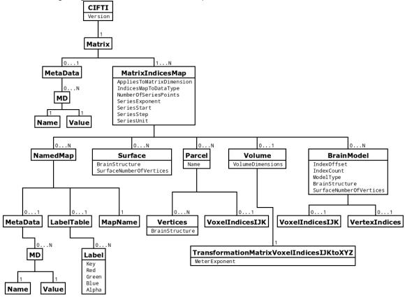
The following diagram shows the relationship between the XML elements in the CIFTI XML.
