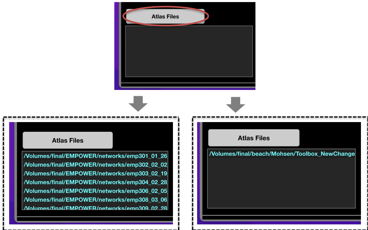
Fig 8. Loading atlas files. You can either select a single atlas file or multiple atlas files. In the latter case, the number of loaded atlas files must be the same as the number of loaded imaging data files, and the number of ROIs must be the same across subjects.
